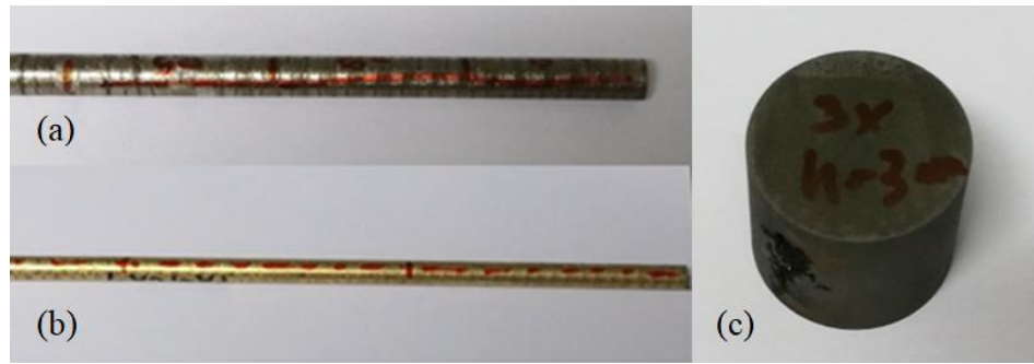
Fig. 1 (a) Ni-Ti CC, (b) Cu-Al-Ni, and (c) Ni-Ti as cast [13].
