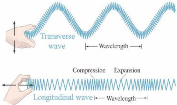
Fig. 3 Illustration of transverse vs. longitudinal waves [7].
