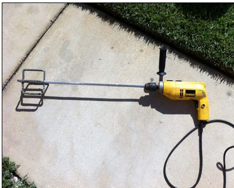
Fig. 1 Due to an unexpected failure of the tank's recirculation pump, the field operator improvised a mixing attempt using an extended DEWALT drill. Although homogenization was not achieved, the RDV® compound remained in contact with the crude matrix under static conditions, initiating a spontaneous reaction that led to measurable transformation over time.
