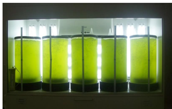
Fig. 1 Laboratory airlift photobioreactors.
