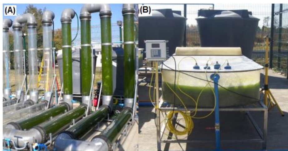
Fig. 2 (A) Tubular airlift pilot photobioreactor, (B) Raceway pilot photobioreactor.
