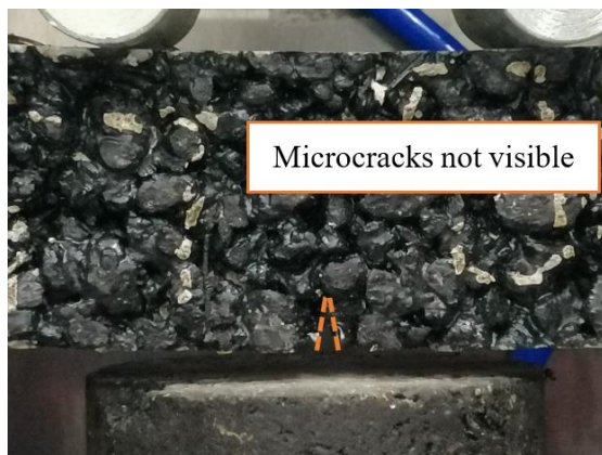
Fig. 10 Early stage under cyclic loading—slight bending (microcracks not visible).
