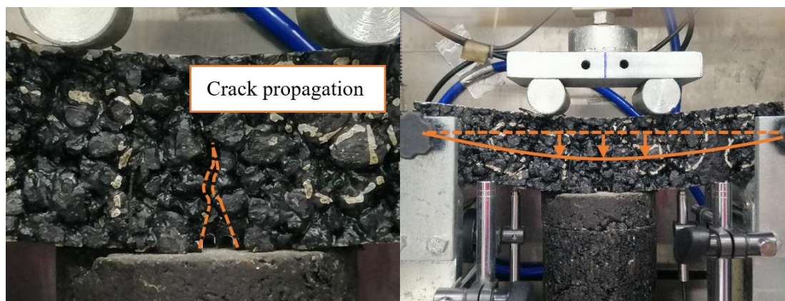
Fig. 12 Crack propagation leading to beam failure.
