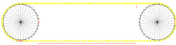
Fig. 2 Simulation model of conveyor chain.
